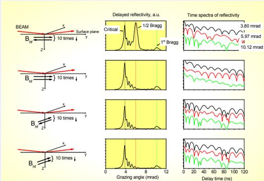
The nuclear resonance reflectivity (NRR) measurements include the angular dependency of the delayed signal + time spectra of reflectivity measured at different grazing angles and provide us with an exclusive depth-resolved information about the magnetization ordering in multilayers.
