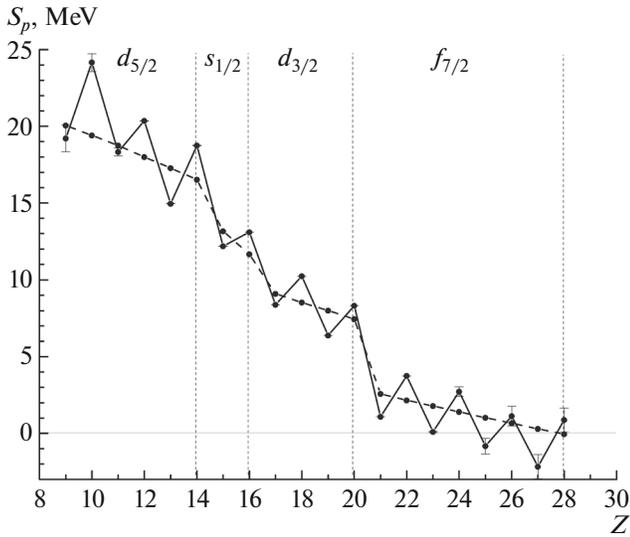
**Fig. 1.** Energy  $S_p(Z)$  of proton separation for  $N = 20$  isotones, derived from the data in [12] on nuclear masses (solid line) and calculated using the SHF formalism (dashed line).
