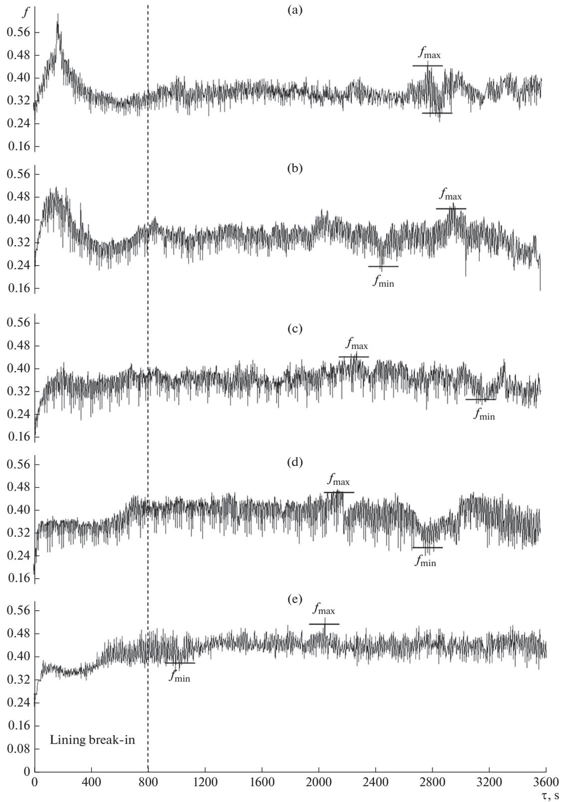
**Fig. 3.** Diagrams of friction tests of (a) as-cast B83 babbitt, (b) hot-pressed B83 babbitt, and CM samples: (c) B83 babbitt + 0.5 wt % MSR, (d) B83 babbitt + 3 wt % SiC, and (e) B83 babbitt + 0.5 wt % MSR + 3 wt % SiC.
