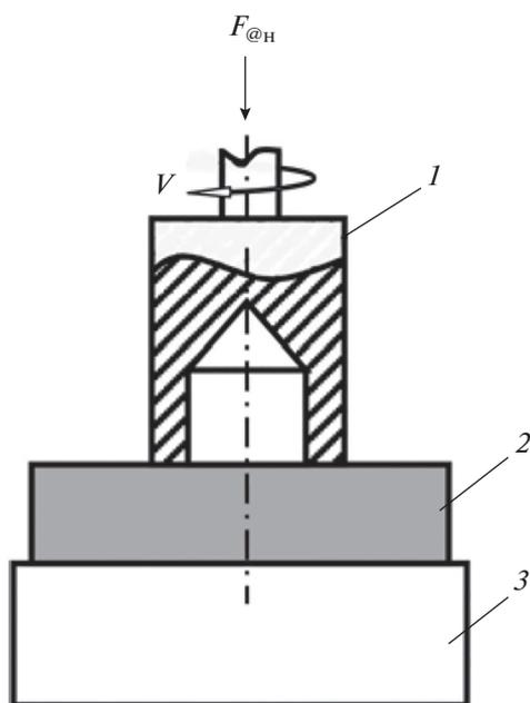
**Fig. 1.** Friction and wear testing setup: (1) grade 45 steel counterface, (2) tested sample, and (3) steel base.
