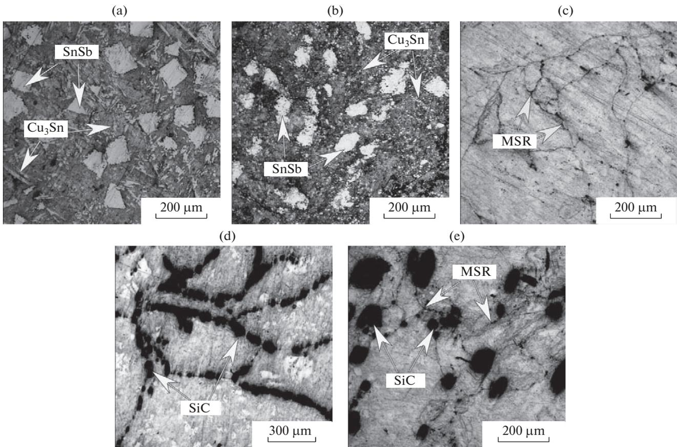
**Fig. 2.** Microstructure of chemically etched (a) as-cast B83 babbitt and (b) hot-pressed B83 babbitt. Surfaces of CM samples: (c) B83 babbitt + 0.5 wt % MSR, (d) B83 babbitt + 3 wt % SiC, and (e) B83 babbitt + 0.5 wt % MSR + 3 wt % SiC.
