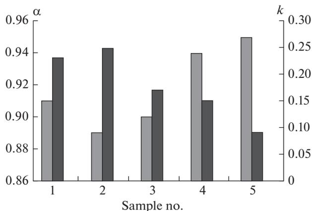
Fig. 4. Friction stability and sustainability coefficients  $\alpha$  (■) and  $k$  (■) of studied samples nos. 1–5.
