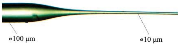
Figure 9. Microscopic view of optical fiber microcontraction
