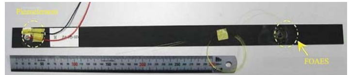
Figure 8. Test composite plate for FOAES
