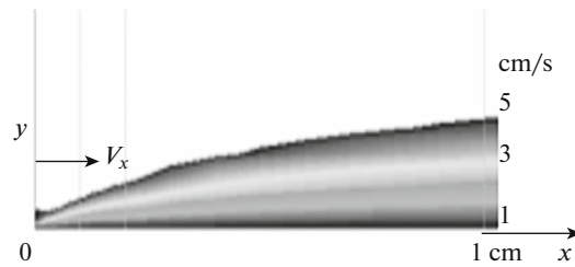
Fig. 2. The hydrodynamic boundary layer near horizontal plate at an initial velocity of the inflow V_{xo} = 5 cm/s: velocity isolines and vertical scale of V_x on initial plate part x \leq 1 cm.
