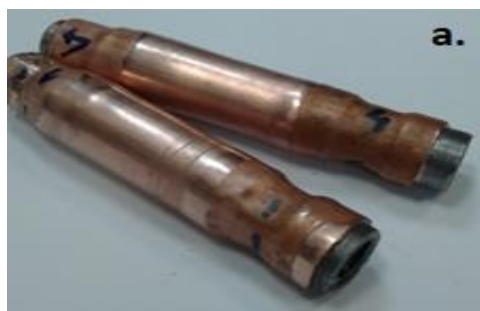
Fig.2. General view of samples after MPCP, drawing and sintering at a temperature of 900°C. Diameter- 16 mm and length- 50 mm.
