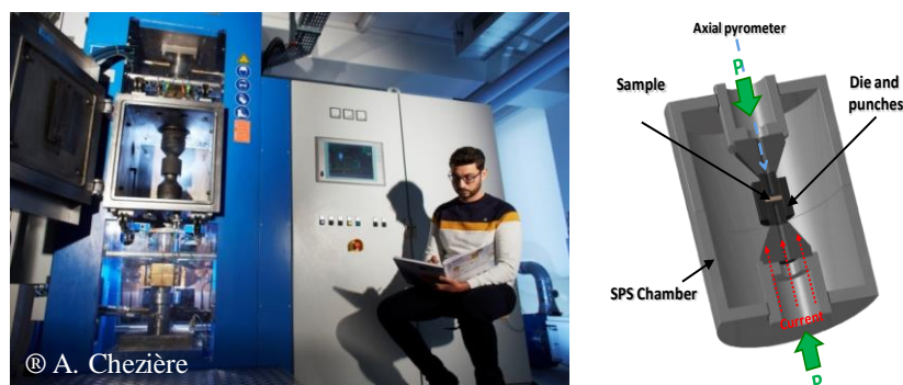
Fig. 1. Left: General view of SPS, Right: Schematic description of the SPS chamber.
