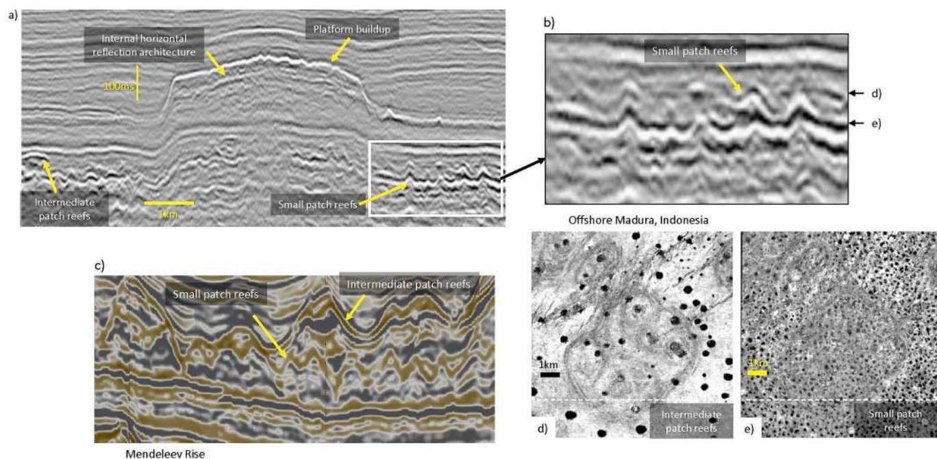
**Fig. 5.** Comparison between Miocene carbonate buildups (a, b, d, and e) from offshore Madura, Indonesia (Posamentier et al., 2010) and c) Mendeleev interpreted buildups (line location shown in Fig. 4). 3D seismic time slices (d and e) through small patch reefs shown in section view (a and b) with numerous small patch reefs (d) evolving into larger patch reefs (e) through time before culminating in significantly larger, higher-relief platforms (a).
