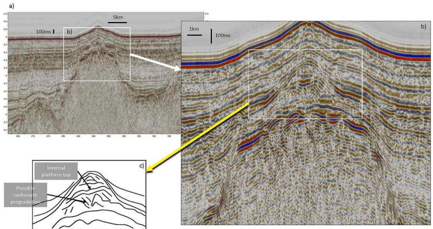
**Fig. 6.** a) seismic section (arc12-03) illustrating carbonate buildups from the Mendeleev Rise (see Fig. 1 for location). b) Detail of the seismic section highlighting the interpreted shallow-water carbonate deposits. c) Interpretation of the detailed seismic section focused on the shallow-water carbonates. Note the internal platform top inferred from the internal horizontal reflections.
