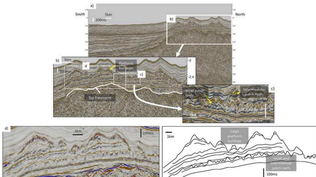
**Fig. 4.** a) Multi-channel seismic section (arc20-24) across the Mendeleev Rise (see Fig. 1 for location). b) Detail of interpreted carbonate buildups illustrating various size patch reefs and platforms. c and d) Detailed view of interpreted small and intermediate patch reefs characterized by small patch reefs at the base, culminating in larger platforms at the top, uninterpreted and interpreted.
