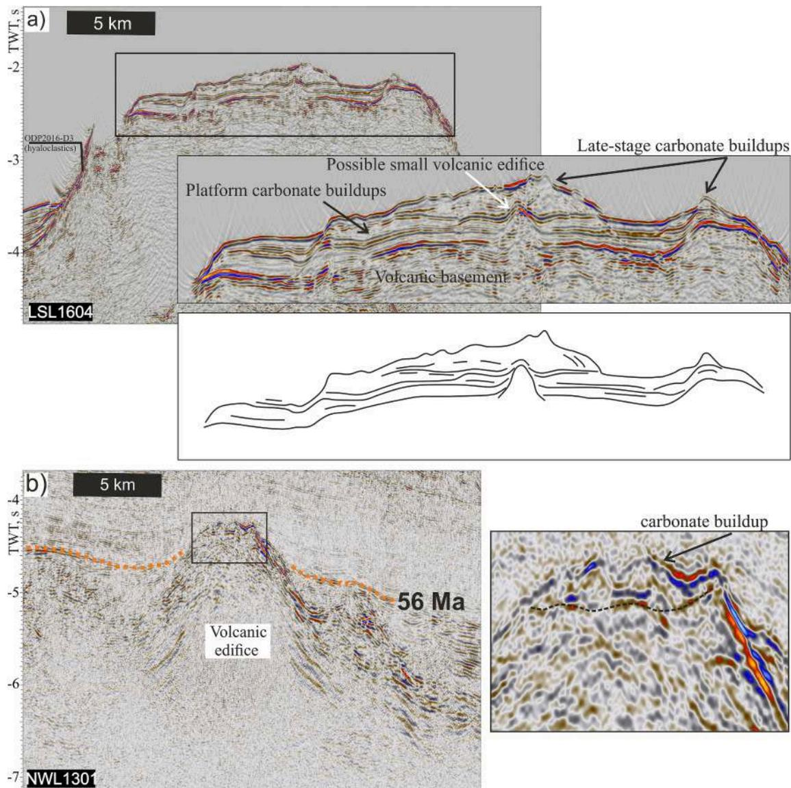
**Fig. 8.** a) Alpha ridge with Fedotov Cretaceous Volcano and carbonate cap. Seismic section from [Funck and Shimeld \(2023\)](#) with our interpretation of shallow-water carbonates. b) Laptev Sea continental slope and Paleocene volcano with possible carbonate cap (See [Fig. 7](#) for location).
