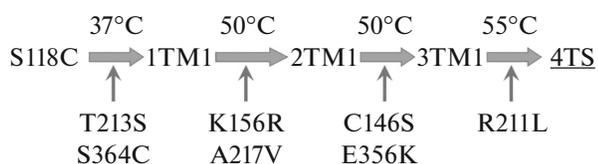
**Fig. 11.** Scheme for obtaining a thermostable mutant of *L. mingrelica* luciferase using the directed evolution method.
