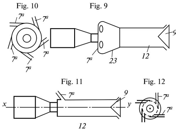
Fig. 2. Multi-input options proposed by Ranque (fragments of the patent FR 743111).
