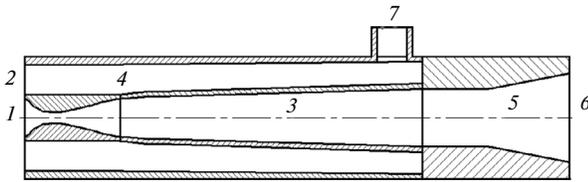
**Fig. 17.** The principal scheme of the device for gasdynamic stratification: 1, entrance to supersonic channel; 2, entrance to subsonic channel; 3, supersonic channel; 4, subsonic channel; 5, diffuser; 6, exit from supersonic channel; 7, exit from subsonic channel.
