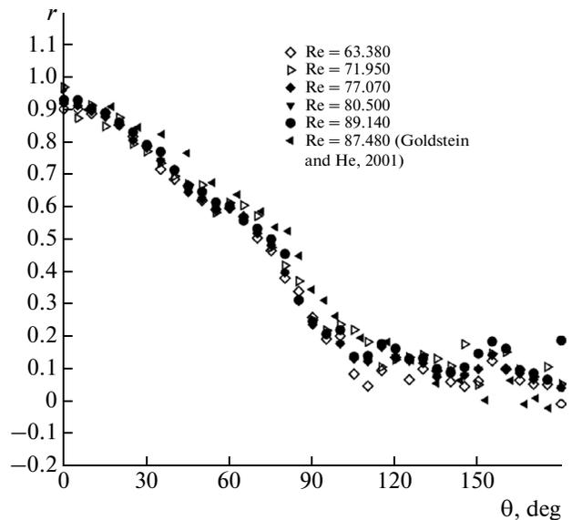
Fig. 13. Variation of the restoring coefficient of temperature over the circumference of the cylinder around which the flow of gas flows [41].
