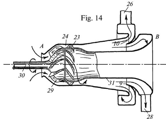
Fig. 3. Mechanical swirler options proposed by Ranque (fragments of the extra patent FR 43164E).
