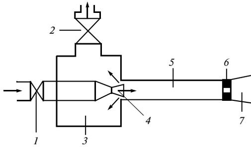
Fig. 7. The ejector with a negative value of the ejection coefficient [26, 27]: 1, 2, regulating taps; 3, antechamber; 4, supersonic nozzle; 5, mixing chamber; 6, diaphragm; 7, diffuser.
