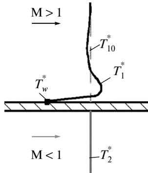
**Fig. 18.** Schematics of the gas dynamic stratification of temperature in the case  $Pr < 1$ .
