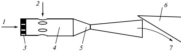
Fig. 9. Scheme of the energy separation device in a two-phase flow [30]: 1, input of water; 2, input of gas; 3, pulverizer; 4, mixer; 5, supersonic nozzle; 6, separator; 7, output of gas.
