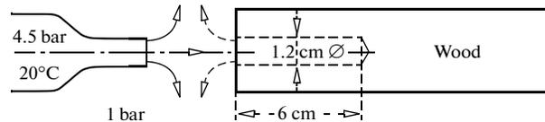
Fig. 5. Scheme of the working part of Sprenger's resonance tube [22].
