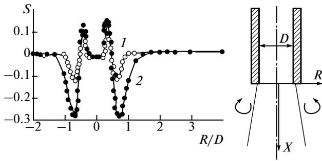
Fig. 14. Stratification in the flow of gas (at the distance  $X/D = 2$ ) [42]: 1, laminar flow; 2, turbulent flow.
