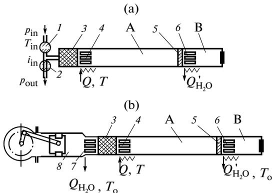
Fig. 10. Improved designs of pulsating tube [36]: (a) with valves; (b) with piston attached; 1, 2, input and output valves; 3, regenerator; 4, heat exchanger-cooler; 5, nozzle (throttle hole); 6, refrigerator; 7, end refrigerator; 8, compressor-expander; A, working space of the tube; B, receiving vessel.
