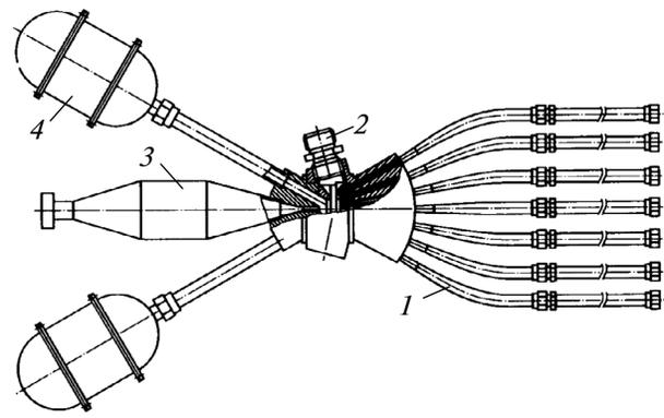
Fig. 11. Structural scheme of the pulsation tube [37]: 1, receptor tubes; 2, input transfer tube; 3, output transfer tube; 4, resonator chambers.
