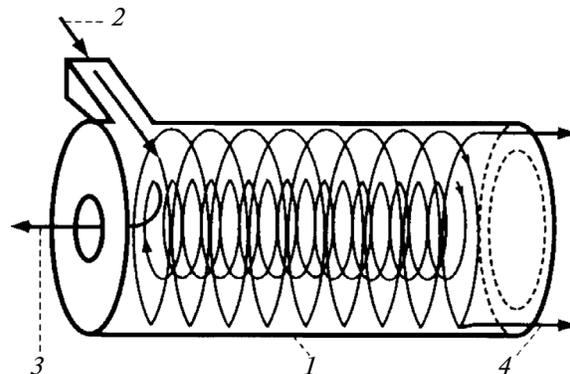
Fig. 4. The picture of the gas flow in a counterflow vortex tube: 1, vortex tube; 2, input of compressed gas; 3, output of cold gas; 4, output of the heated flow.
