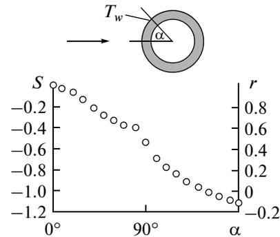
Fig. 12. Parameter  $S$  and coefficient  $r$  of temperature restoring on the surface of a cylinder around which the flow of gas flows [38].
