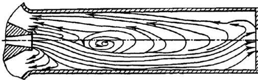
Fig. 8. Scheme of the gas flow in a mixing chamber of the ejector with a negative value of ejection coefficient (right, output of hot gas; left, input of compressed gas and output of cold gas).
