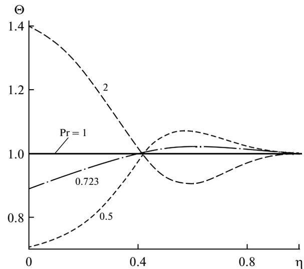
Fig. 16. Distribution of the dimensionless braking temperature for the flow of compressible gas flowing around a thermally isolated wall (for different values of the Prandtl number) [45].
