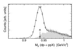
**Fig. 1.** Distribution in missing masses for the  $dp \rightarrow ppX$  reaction for 726 MeV deuterons incident on a storage cell filled with polarised hydrogen. Events that originated from the walls of the cell gave rise to the tail at high  $M_X$ . The shape of this background was simulated by filling the cell with nitrogen gas and this led to the shaded area. The solid line represents the fit of a Gaussian plus the numerical values of the scaled background histogram.
